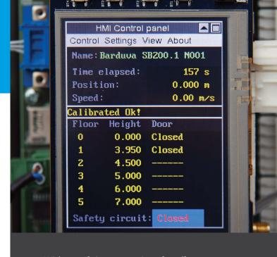
With a sufficient expertise of staff a computer may be used instead of a module to implement the modifications and even reprogram the system completely. The diagnostic module helps to perform the functions of the remote monitoring, voice messaging and two-way wireless speakerphone via GSM.
